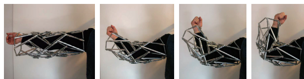
Fig. 16 Movement simulation of joint part of exoskeleton power-assist device using tensegrity structure.
